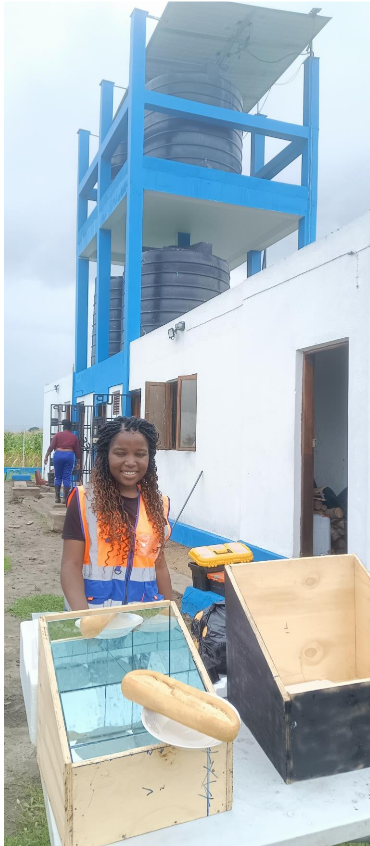
Figure: Homemade solar oven built with readily available (local) materials.
