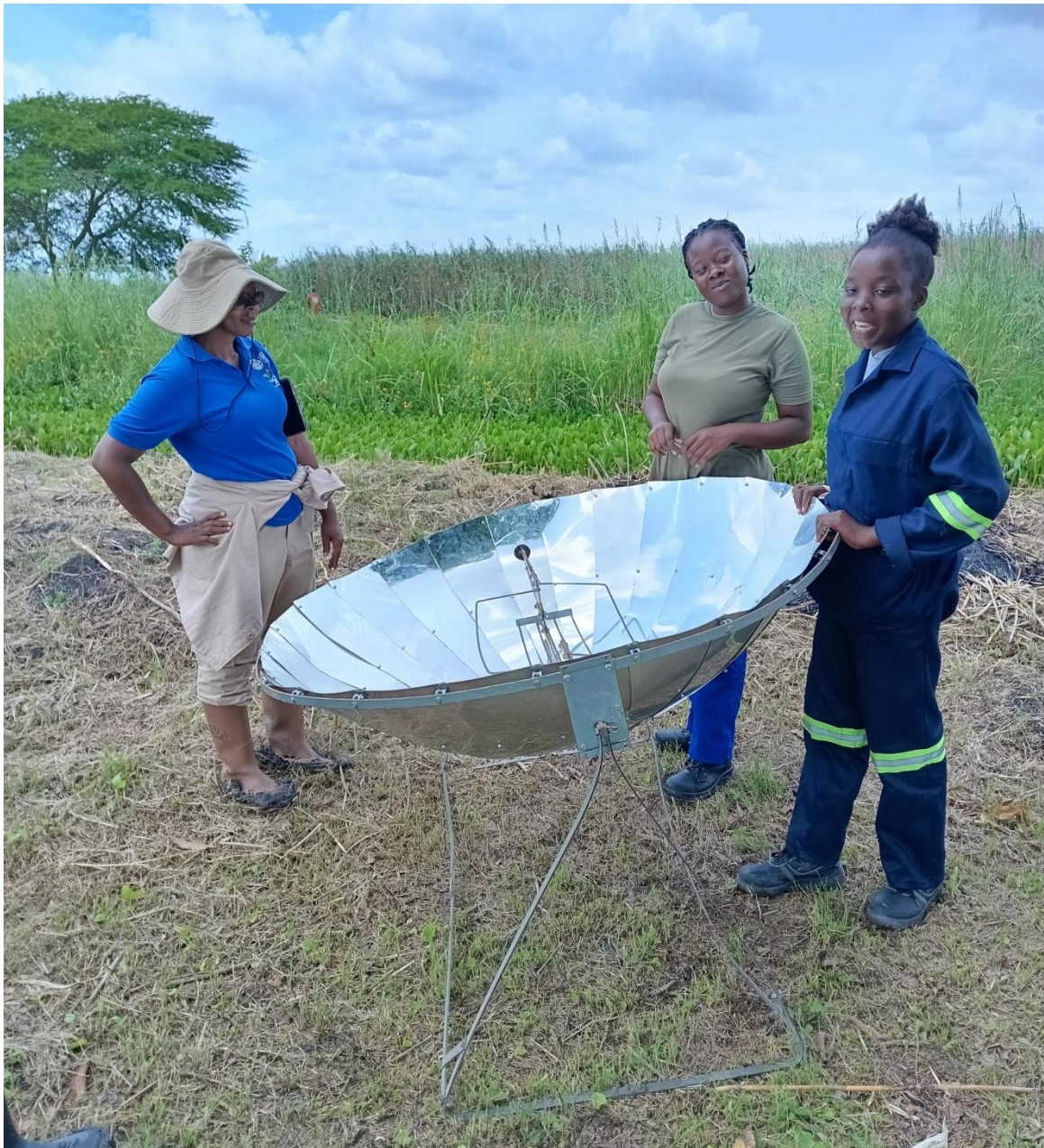
Photo: Solar water heater for heating water and cooking food.
